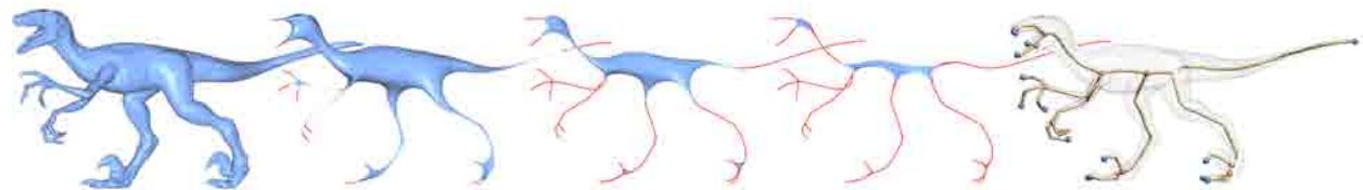
Figure 3: Successive Laplacian smoothing and joint clustering converges to an internal skeleton [Au et al. 2008].
